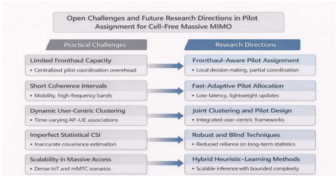
Figure 3: Key open challenges and corresponding research direction for pilot contamination in cell-free massive MIMO system
