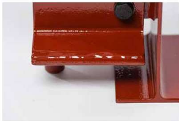
▲ AESS 1: Continuous weld appearance.
