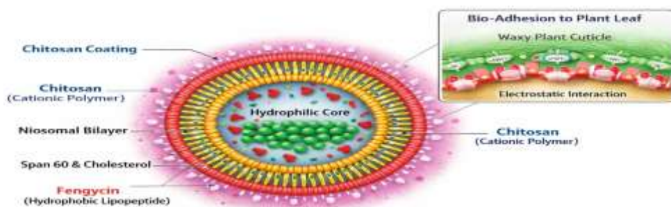
Figure 1: Schematic representation of the Chitosan-coated niosomal system. The design features a hydrophilic core loaded with Surfactin/iturin and a hydrophobic bilayer entrapping Fengycin. The external Chitosan coating provided zeta-potential reversal (cationic charge) to facilitate mucoadhesion to negatively charged plant leaf surfaces.
