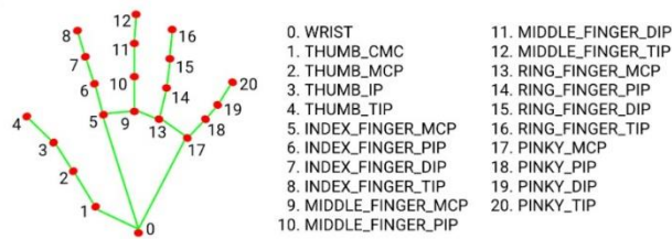
Fig. 2. MediaPipe Hand Landmark Model with 21 Key Points.
