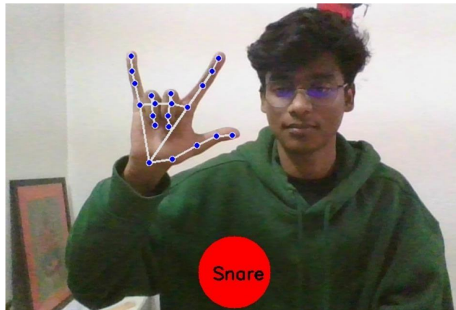
Fig. 6. Real-time gesture recognition and feedback. MediaPipe detects the hand landmarks and classifies the gesture, which is mapped to the “Snare” sound. The corresponding feedback is shown as a labeled animation overlay.
