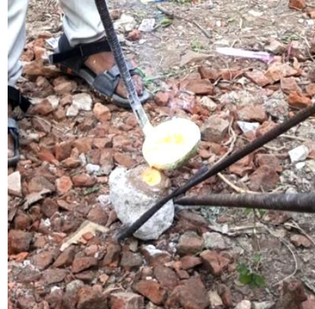
FIGURES 10: Pouring Brass Metal into the Channel (Primary Resource)
