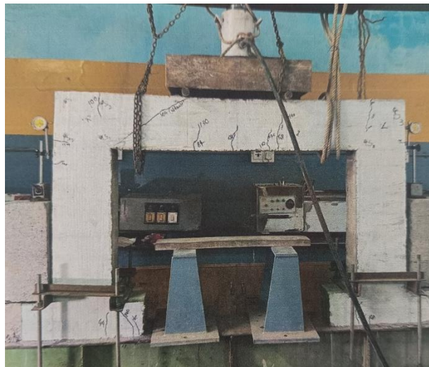
Figure 9: Failure pattern of frame with king cross steel profile
