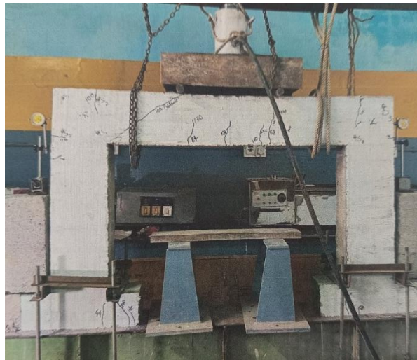
Figure 5: Failure pattern of control frame
