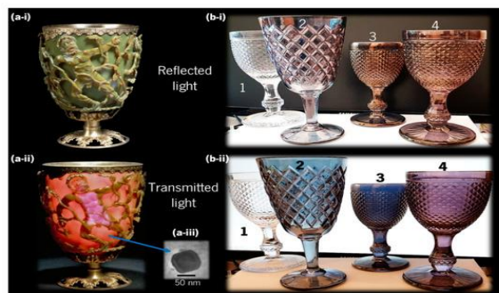
Fig.1 the Lycurgus cup in both transmitted (right) and reflected (left) light Reference. [8]
