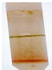
Figure. 4. Chromatography strip obtained using diethyl ether as the solvent system, showing overlapping chlorophyll bands and the absence of a distinct xanthophyll band.
