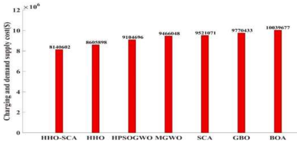
Fig 5 Cost of Charging and demand supply with HHO-SCA, HPSOGWO, MGWO, GBO, SCA, BOA.
