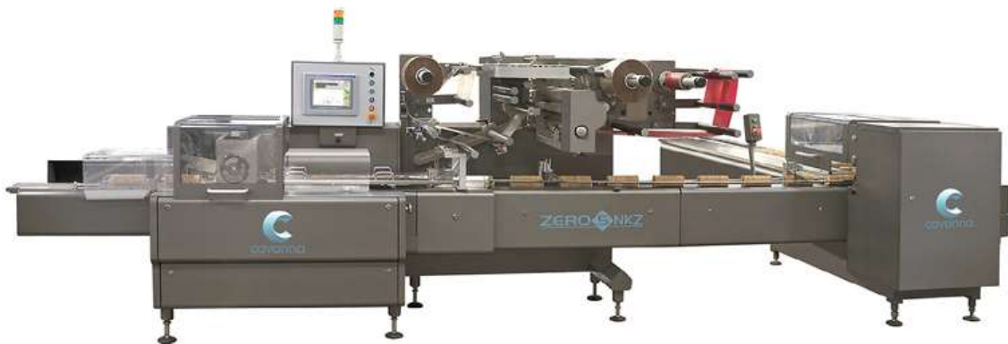
Fig. 7. Cavanna Zero 5 NKZ wrapping machine for slug products with automatic feed.
