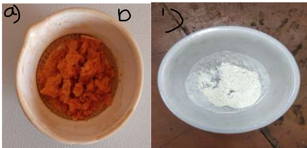
Figure 1: a) Precipitate of ZnO after drying in oven b) ZnO NPs after calcination at 400 degrees
