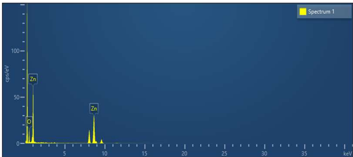
Figure-6: EDX Spectra of ZnO NPs
