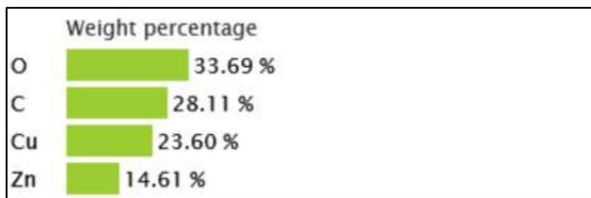
Figure 10.3. EDX Analysis of the Elemental Composition of the Cu-Zn Nanoparticles for V3.
