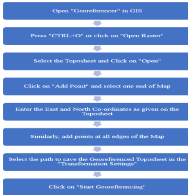
Figure 5: Process of Georeferencing of Toposheet
