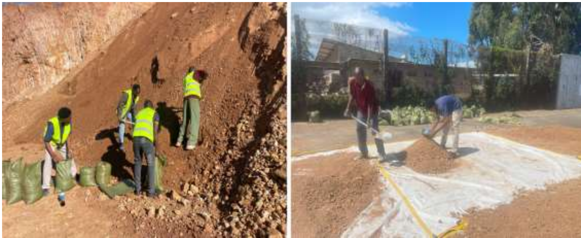
Figure 1: Photo of excavated materials at borrow pit (left) and air dried at lab (right)
