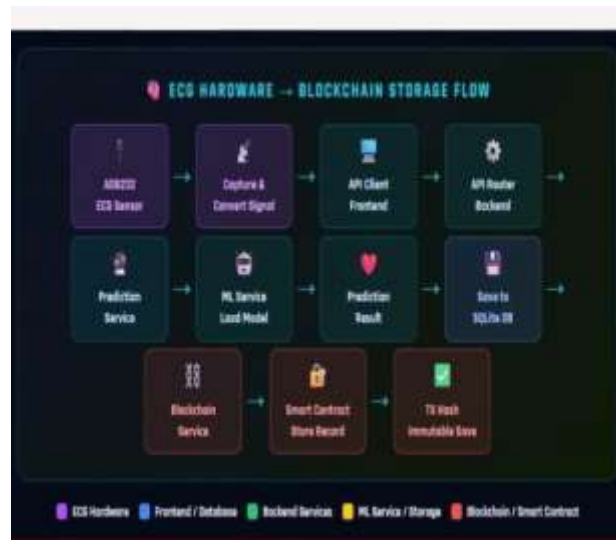
Fig. 2. End-to-end flow: ECG hardware → capture & convert signal → API client frontend → API router backend → prediction service → ML service (load model) → prediction result → save to SQLite DB; optional path via blockchain service → smart contract (store record) → transaction hash (immutable save). Data is taken at the point of care, handled by a central backend, written to SQLite for fast access, and optionally sent to the chain for a tamper-evident trail [7], [8].
