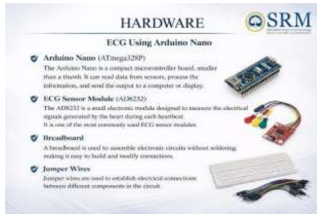
Fig. 1. Hardware components for ECG data acquisition using Arduino Nano: Arduino Nano (ATmega328P), AD8232 ECG sensor module, breadboard, and jumper wires.
