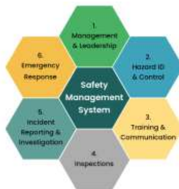
Figure 11: Elements of the safety management system (Elements of the safety management system - Search Images)
