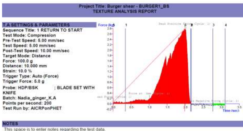
Graph 4: The graph shows the test of compression using HDP/BSK blade on ginger variety Nadia where Force (Kg) is analyzed with time.
