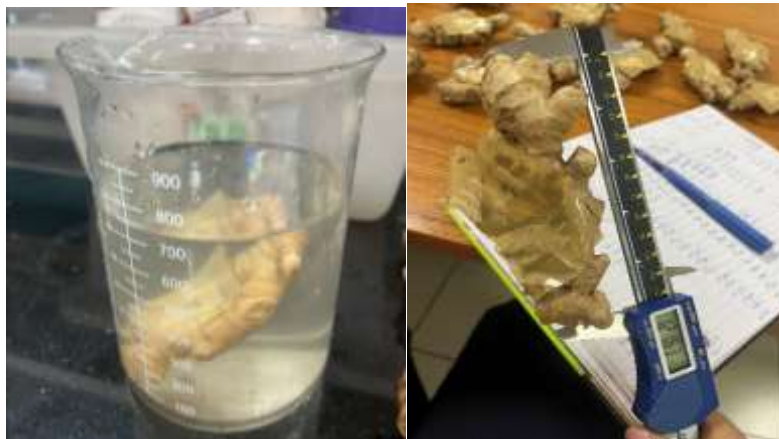
Plate 2: Shows the use of a digital Vernier caliper to measure axial dimensions in Jorhat, Assam.
