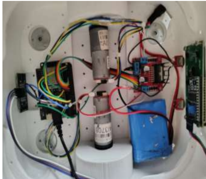
Fig3. Motor driver and control circuitry implementation
