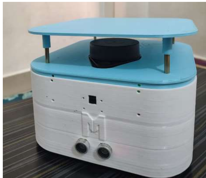
Fig4. Mechanical structure and LiDAR placement carrying capability
