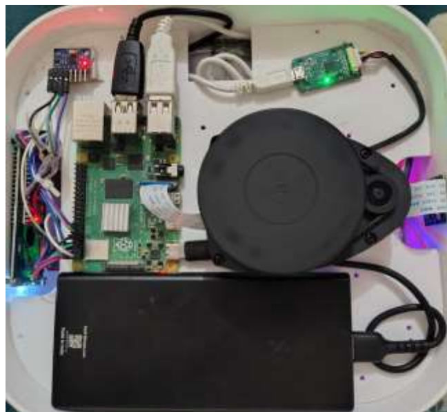
Fig2. Internal electronics layout of the proposed robot system
