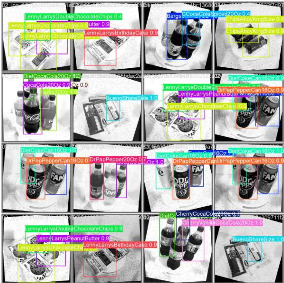
Fig. 6: Multiple object detection in a single image, which demonstrates the system’s ability to detect more than one object in a single image.
