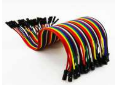
Fig:7 Jumper wires
