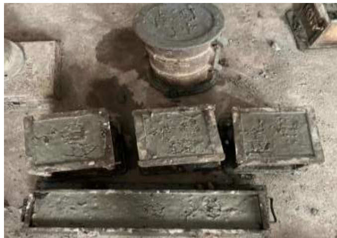
Drying of Moulds after Casting
