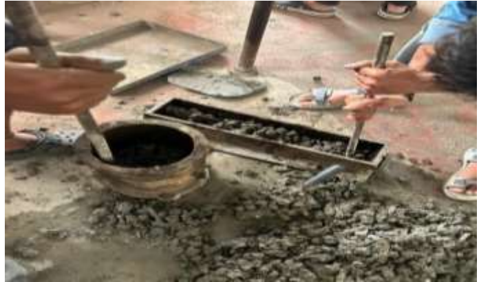
Casting of Cubes, Beams and Cylinders
