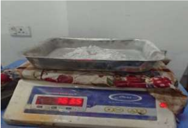
Weighing of Cement
