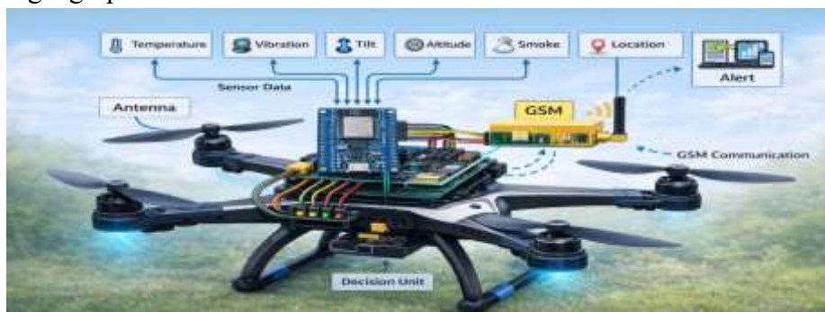
Figure 7: Embedded monitoring system architecture with sensor interfacing and GSM communication
