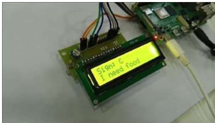
Fig. 6. LCD output for the recognized gesture corresponding to the message “I Need Food”.
