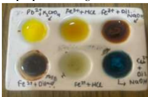
Figure 6: Spot plate showing colour test for cations
