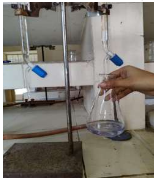
Figure 2: Blue colour (Disodium salt of EDTA solution in burette 2)
