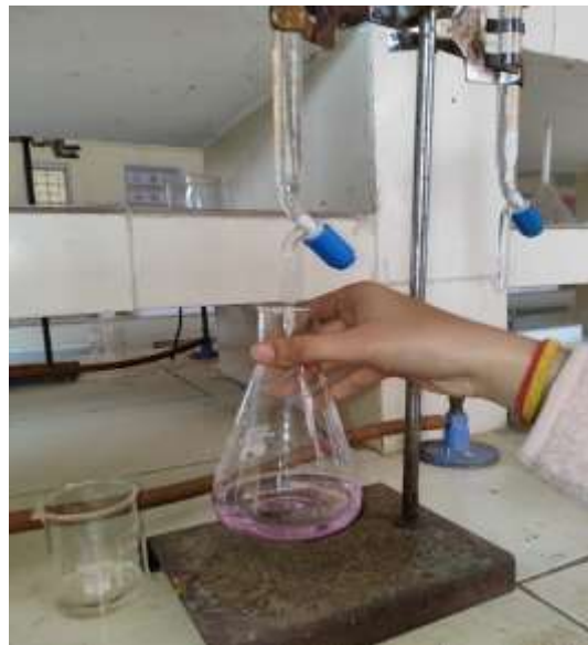
Figure 1: Wine red colour (Magnesium sulphate solution in burette 1)
