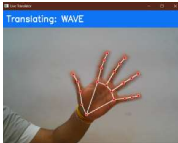
Fig. 5. Real-Time Translation Output — Live webcam feed with MediaPipe landmark overlay, 15-class probability bars, system info panel, and stabilized translation label in the header banner.
