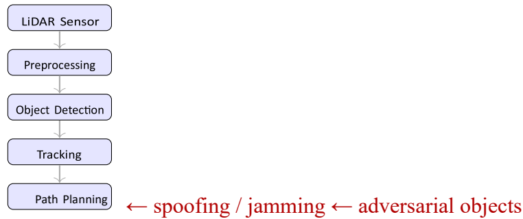
Fig. 2. Figure 2: Autonomous vehicle perception pipeline. Red labels show attack entry points: signal-level attacks corrupt the sensor; adversarial objects exploit the detection stage.
