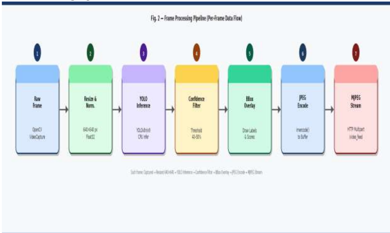
Fig. 2 — Frame Processing Pipeline: Raw Frame → Resize & Normalise → YOLO Inference → Bounding Box Annotation → MJPEG Stream Output
