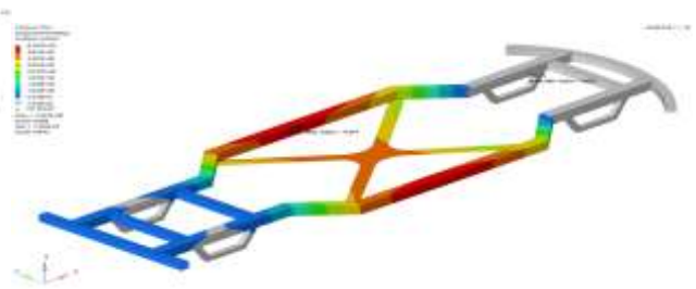
Deformation of conventional steel
