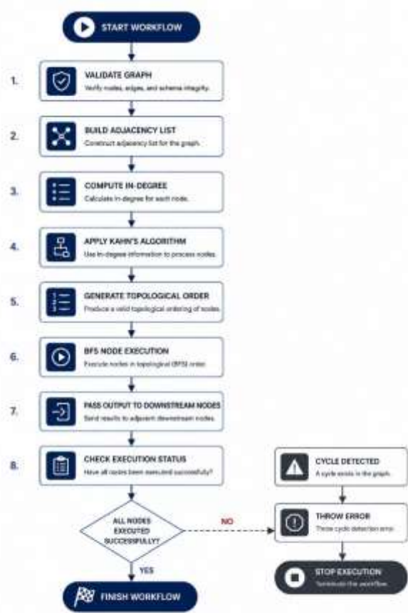
Fig. 1. Workflow execution process in the automation platform using topological sorting and BFS-based node execution.
