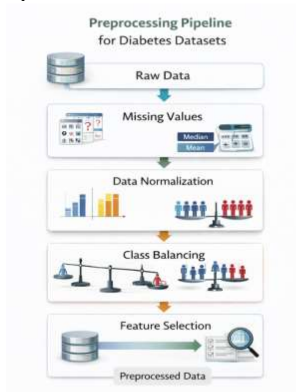
Fig. 3. Overview of the data preprocessing and feature engineering pipeline used in diabetes prediction studies.
