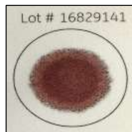
Figure 06: FTA Card containing a blood sample, isolated DNA preserved for several days for further DNA analysis. [12]
