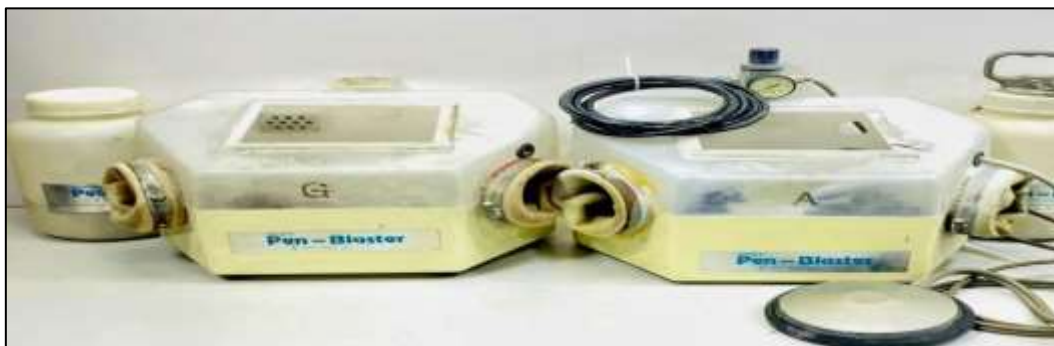
Figure 3: Pen Blaster (Shofu) used for Sandblasting of fiber post with 50 mu size of Aluminium Particle.
