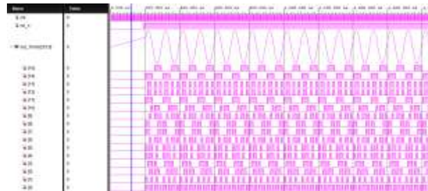
Figure 4: Behavioral simulation capturing the generated Continuous Direct Digital Synthesis (DDS) raw bitstreams.
