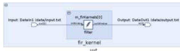
Figure 3: Vitis Analyzer Graph View showing the synthesized an AI Engine tile mapped to fir_sr_sym filter kernel successfully, PLIO streams routing via input.txt and output.txt.
