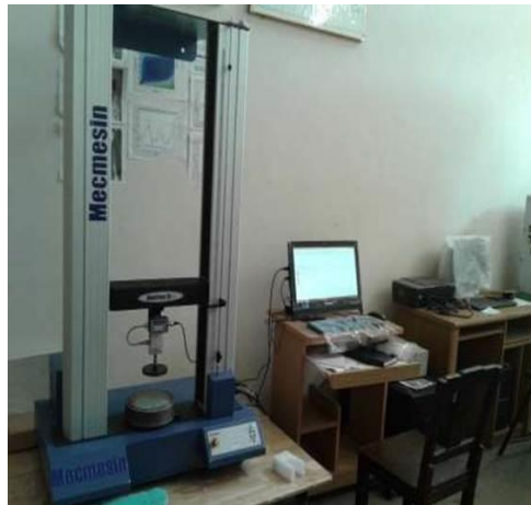
Fig 4: Nano Material testing Machine connected to automatic data acquisition system
