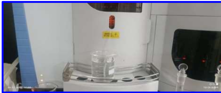
Fig7: Soil sample injected to AAS
