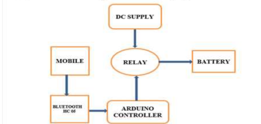
FIGURE 1. Block Diagram of the Charging Protection Circuit
