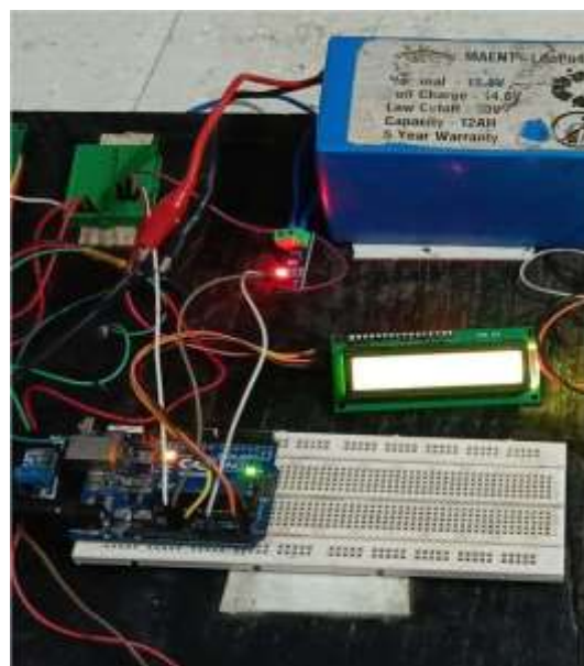
Figure 4: Experimental Prototype for State-of-Charge Measurement Validated on an E-Cycle Pack
