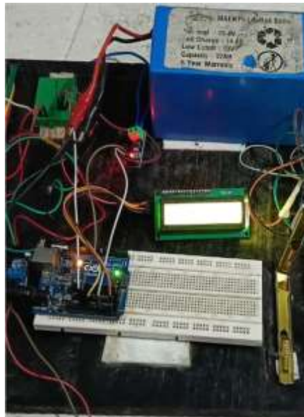
Figure 9: Hardware Prototype for E-Cycle Charging Monitoring
