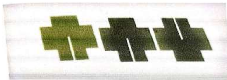
Figure: 1.3 Pre-cut Gafchromic EBT 2 Dosimeter Film
