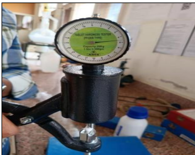
Figure 2: Hardness value ( 4.5 \pm 0.1 \text{ kg/cm}^2 ) of F2 formulation
