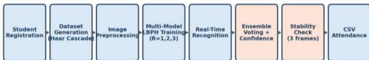
Fig. 1. End-to-end methodology workflow of the proposed AML-LBPH attendance system.
