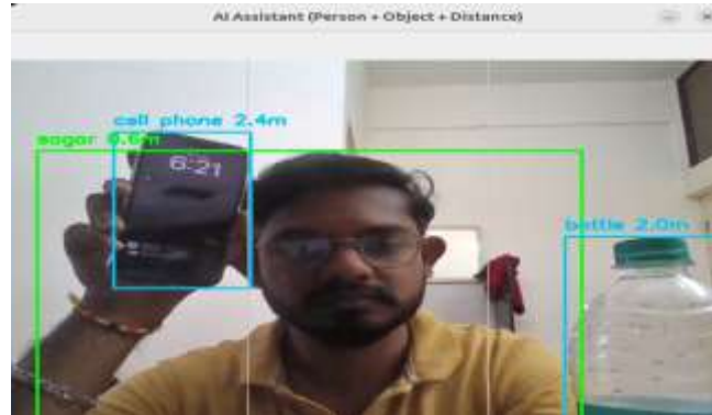
Fig. 4. Detection of multiple objects where a human, cell phone, and bottle are identified at once along with distance estimation.
