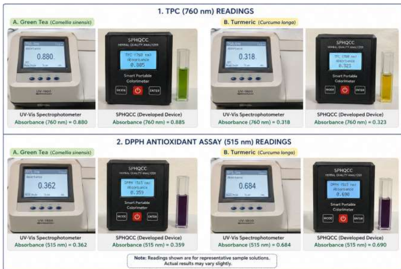
Figure : Representative comparative display of TPC and DPPH assay readings obtained using the developed Smart Portable Herbal Quality Control Colorimeter (SPHQCC) prototype and reference UV–Visible spectrophotometer for herbal sample analysis.
