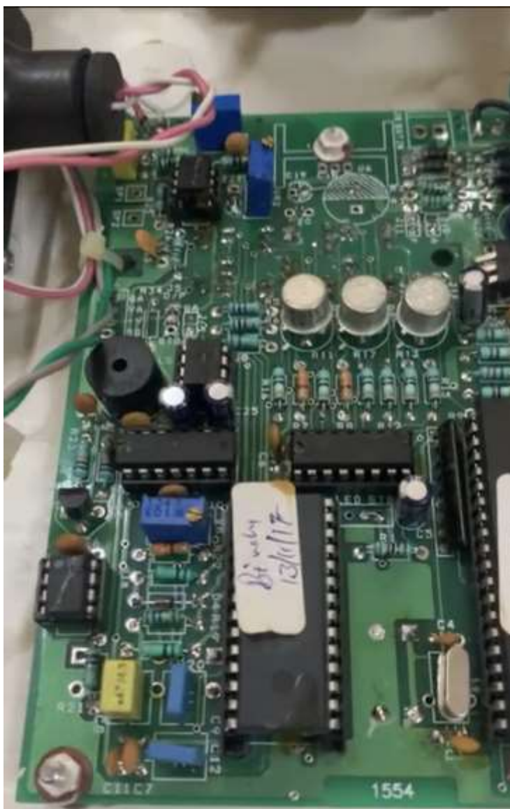
Figure : Internal Printed Circuit Board (PCB) and Signal Processing Circuitry of the Developed SPHQCC Prototype.
