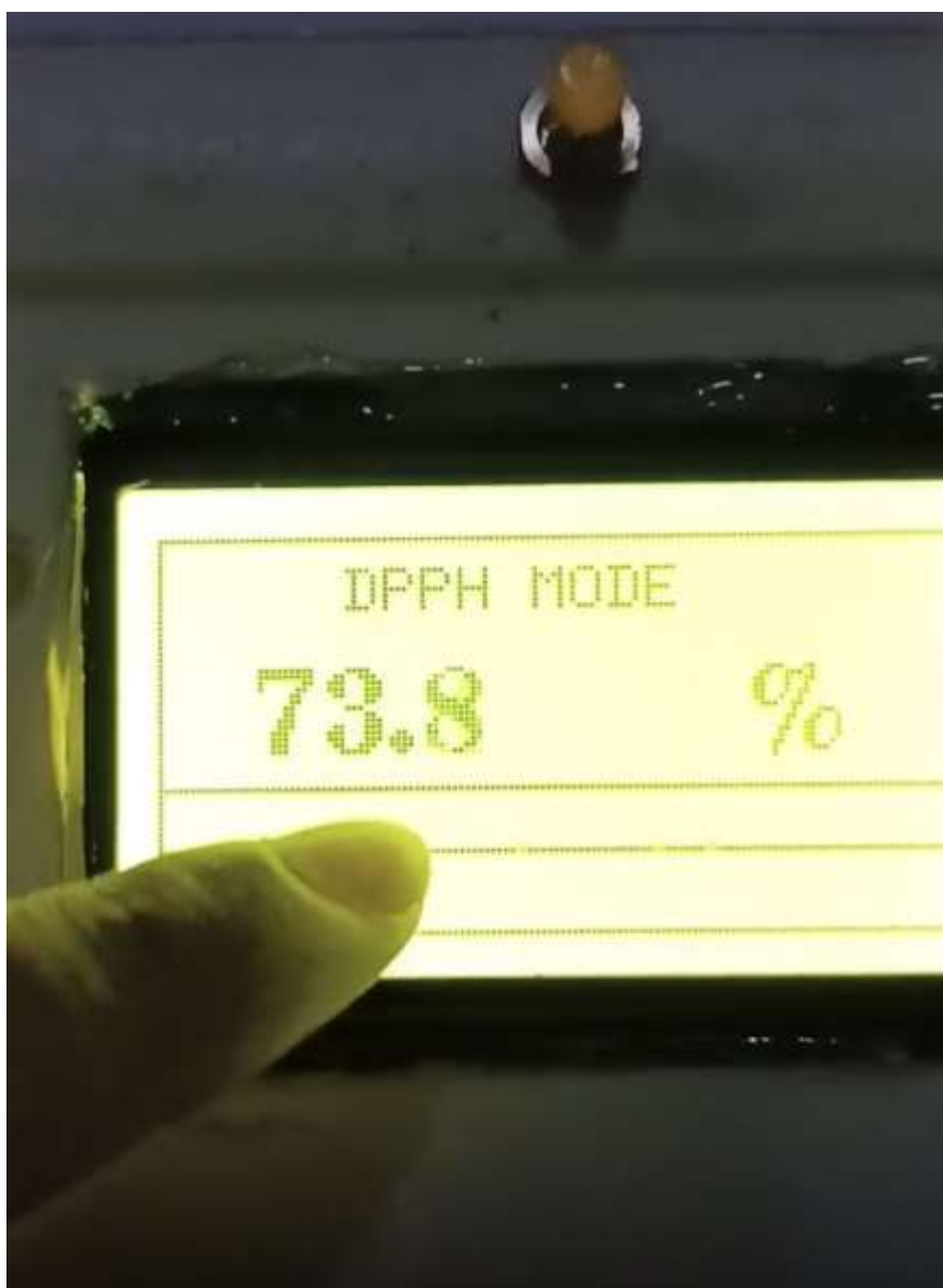
Figure :Digital Display Interface Showing DPPH Antioxidant Assay Mode of the SPHQCC Prototyp.
