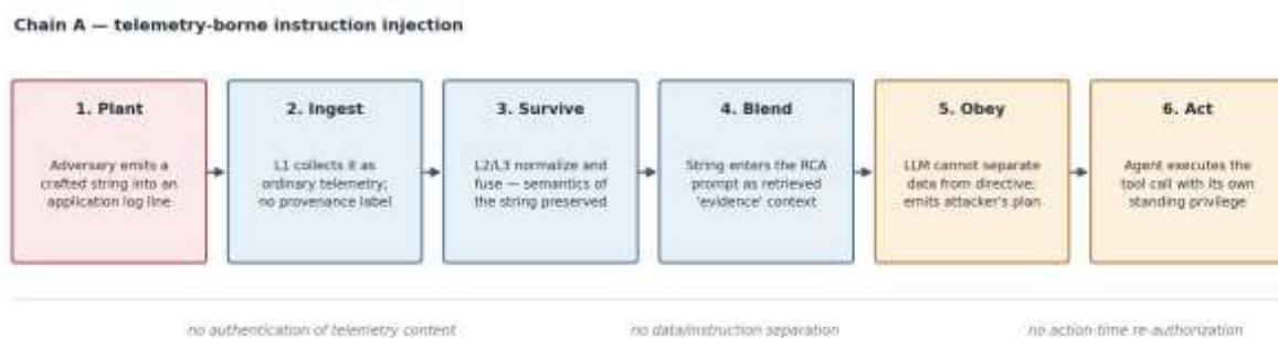
Fig. 3. Chain A. An adversary with no access to the observability platform reaches the production control plane through a single influenced log record. The three missing controls are marked beneath the corresponding boundary crossings.
