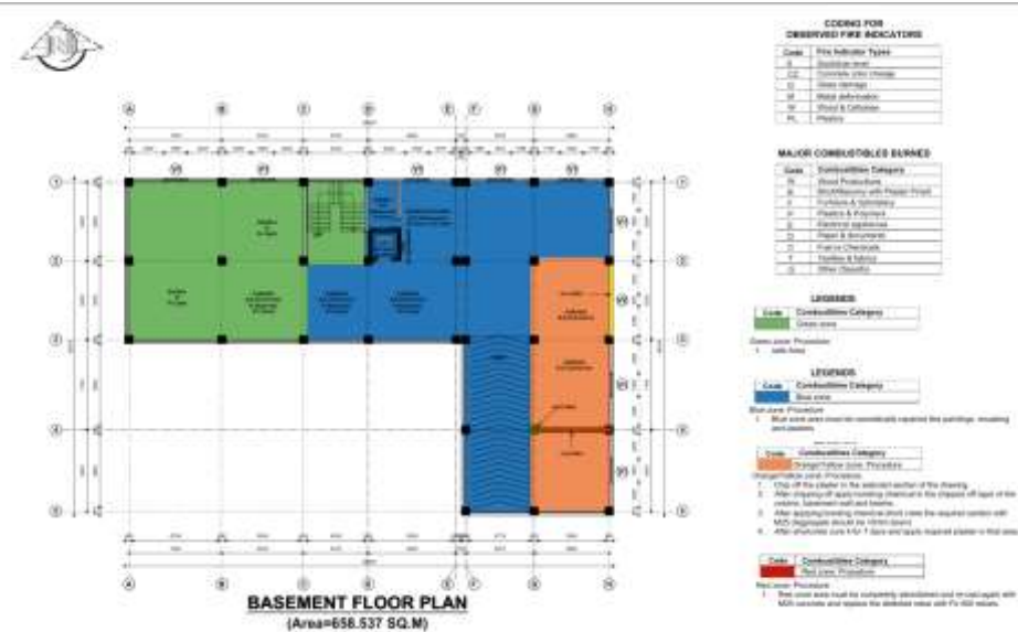
Figure 2: Example of the Mapped Output at Basement Level, Showing Fire Indicator Coding, Combustibles Burned and the Zone-Wise Intervention Required
