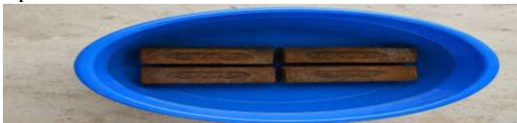
Figure 23: Water absorption test of conventional
