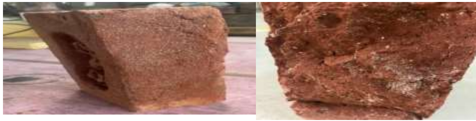
Figure 24: Efflorescence test of conventional brick.
