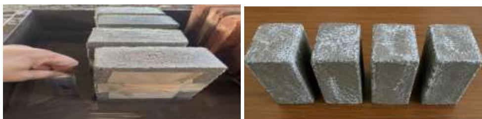
Figure 5 (a)&(b): Efflorescence test of conventional brick.
