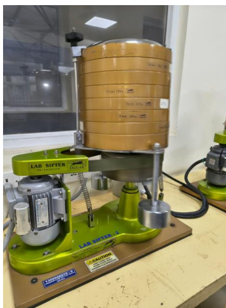
Figure 1. Laboratory Sieve Shaker Used for Particle Size Fractionation of Ragi Flour
