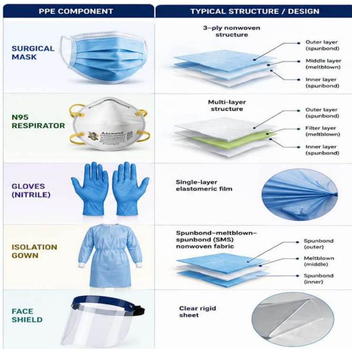
Figure 2 : PPE components and their structure
