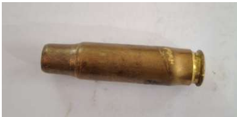
Figure 6: It shows bulging in the lower portion of the empty cartridge case, which was fired using the modified .303" British rifle, indicating improper chamber conformity.
