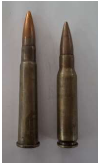
Figure 1: It shows the types of ammunition used in this examination - .303" (7.7 x 56 mm) caliber cartridge, and 7.62 x 51 mm caliber cartridge (up to down)
