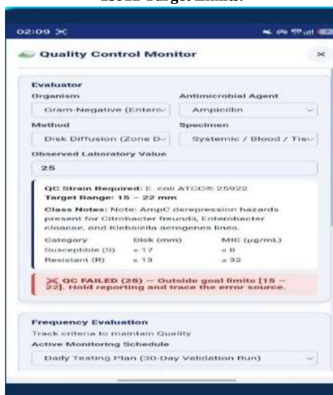
Figure 5.1 Real-Time QC Monitor Flagging an Out-of-Range Disk Diffusion Result Against ATCC 25922 Target Limits.
