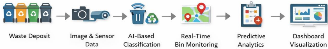
Figure 2: Workflow of the Proposed AI-Based Waste Management System
